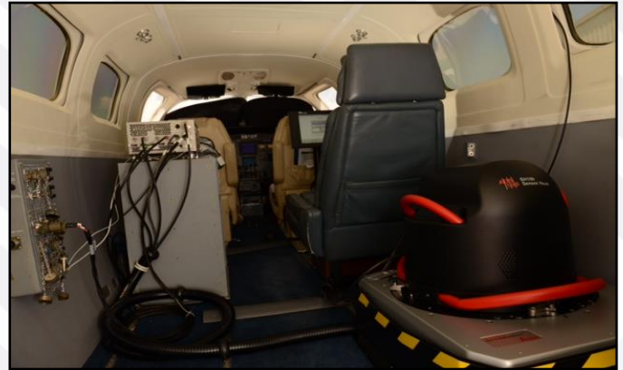
Leica ADS100 installation in a Cessna 441 (Conquest)
