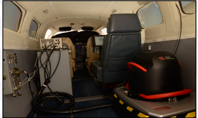
Leica ADS100 installation in a Cessna 441 (Conquest)
